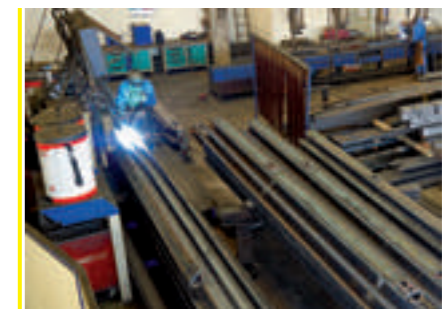
longitudinal welding station
